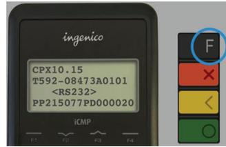
If the Functions menu is not displayed, you can reboot the terminal by holding the power button, and try again.
