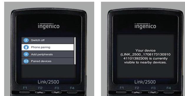
Use the **F2** and **F3** keys to move your selection up and down. The pairing process requires that you enable Bluetooth on your mobile device.
